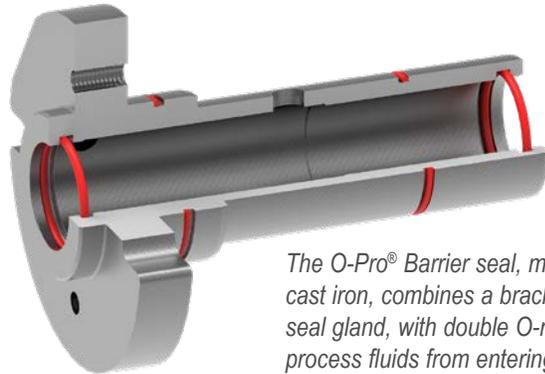
*The O-Pro® Barrier seal, made of hardened cast iron, combines a bracket bushing and seal gland, with double O-ring seals, to stop process fluids from entering the bracket and eventually leaking from the pump.*
