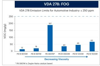
The low emission profile for mPB-1 is a direct result from the solution polymerization technology used for the production of PB-1 where Butene-1 is not only the monomer but also acts as the solvent. Hence, the process is rather clean as it avoids the use of any external high molecular weight solvent. The combination of metallocene technology providing a precise control over the polymer structure and the efficient finishing section in the production ensures adequate residual monomer.
