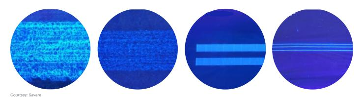
Above spray patterns show a very precise glue path offered by the *Koattro PB M 1500M* ensuring superior production efficiency.
