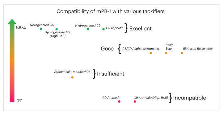
Compatibility of mPB-1 with various tackifiers using cloud point method in a formulation comprising of 70% Polymer and 30% tackifier. 'Cloud Point' is the temperature at which the hot melt adhesive becomes cloudy upon cooling from melt and is a measure of compatibility of the formula components.
