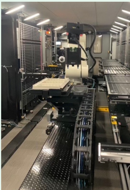
Inside of the Omnicell XR2 Robot at Mercy Health — St. Rita's Medical Center.
