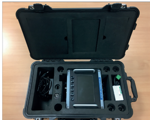
The equipment is contained in a small case: 54cm (21in) (l), 36cm (14in) (w), 22cm (9in) (h) and weighs 15 kg (33lbs). A standard unit is composed of one data-logger, a set of pressure transducers with different pressure ranges, cables and chargers. The equipment is ATEX Zone 2 and contains a 65Wh lithium-ion battery.
