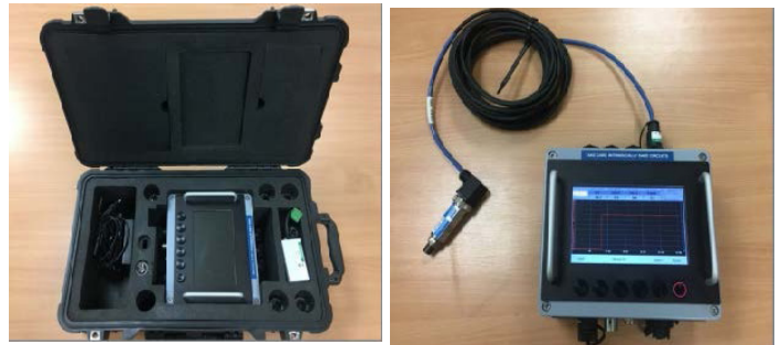
InnerVue™ diagnostic equipment, including pressure transducers (with different ranges), data-logger, cables and charger.
