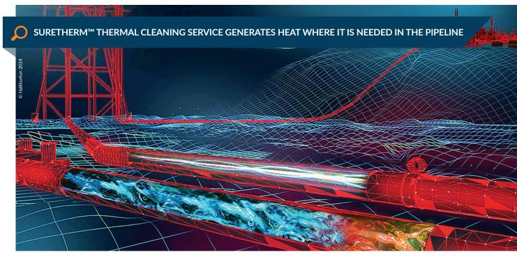
When paraffin wax builds up in oil and condensate pipelines, operators have several options to remove the blockage. One of the options to clear the blockage is using solvent-based paraffin treatments which are typically most effective when applied at elevated temperatures. In low temperature environments like subsea, however, the ability of solvents to remove significant quantities of paraffin is reduced.
