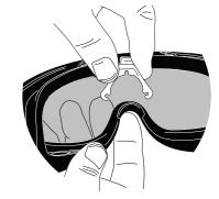
Separate the frame from the top of the lens. Grab exposed lens and pull the lens from the goggle frame.
