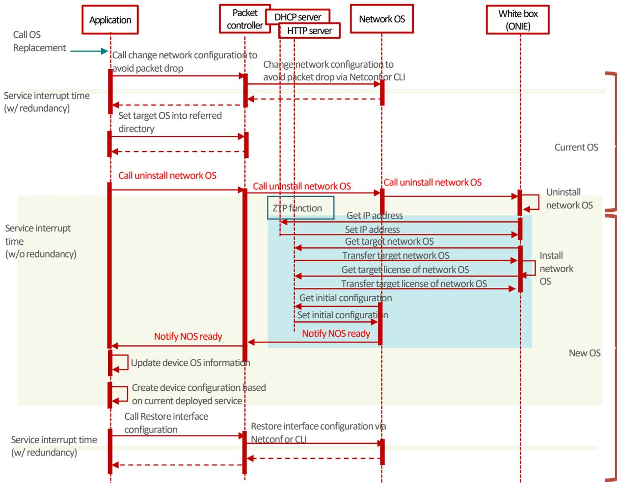
Figure 2. Workflow for automatic NOS replacement procedure
