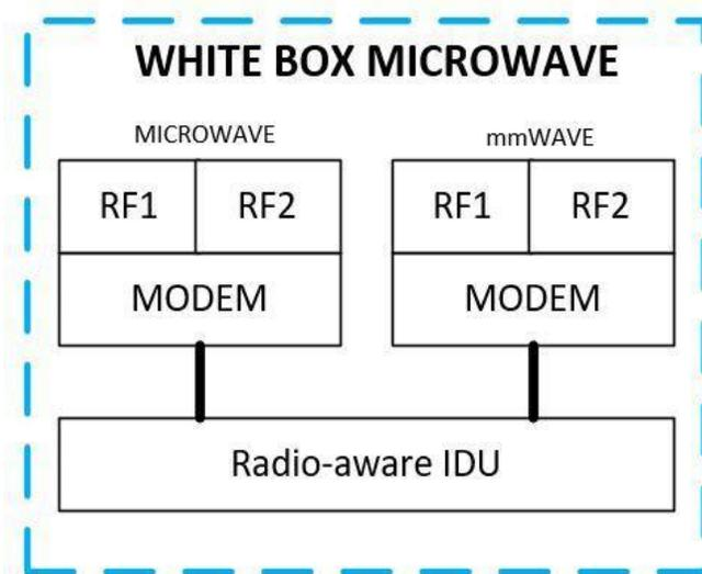
Figure 6 - Open MW Platform High-Level Architecture Components
