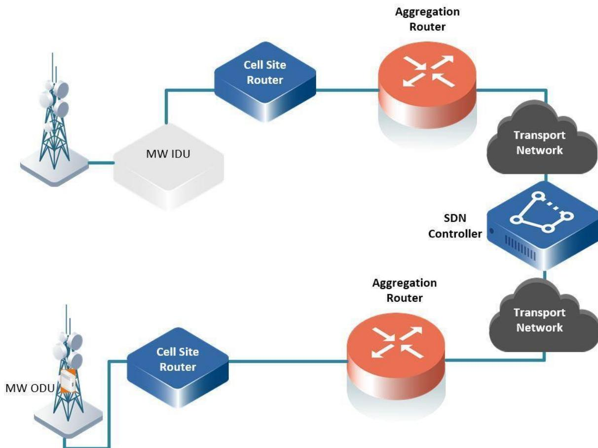
**Figure 10 - SDN Controller Connectivity Architecture**
