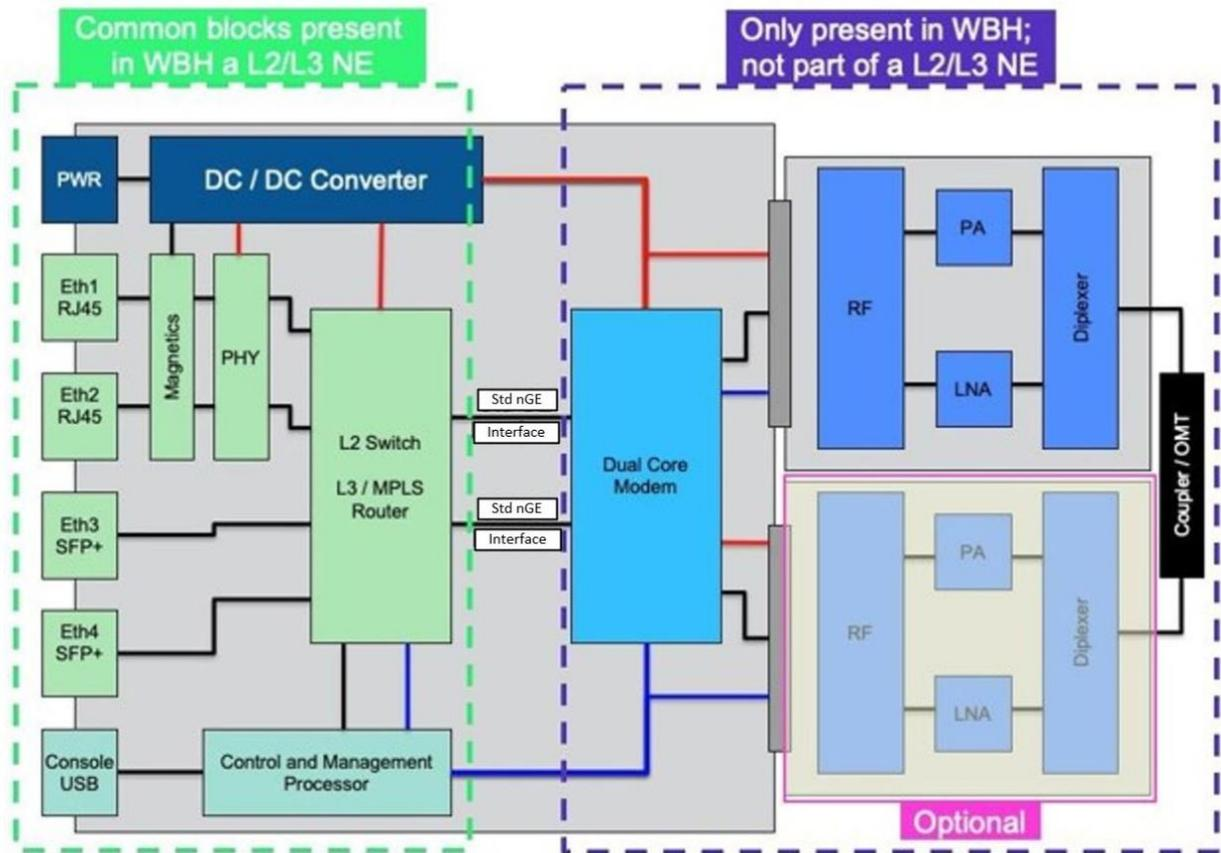
Figure 2 - System Architecture
