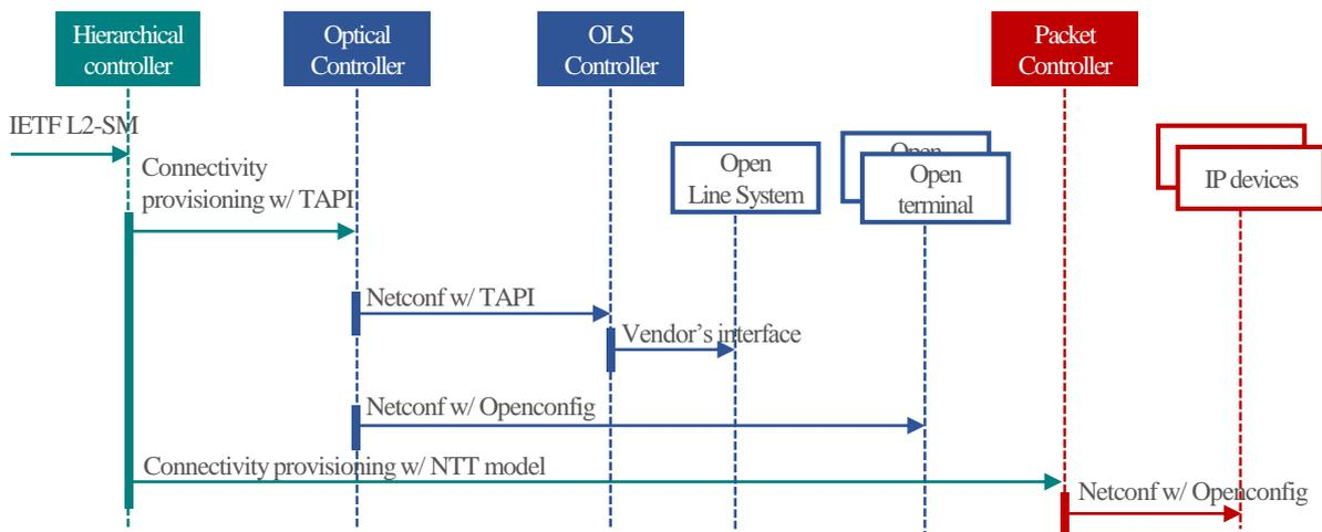
Figure 4. End-to-end provisioning workflow
