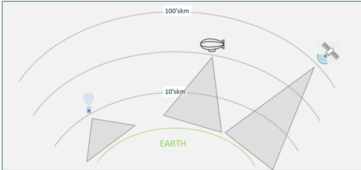
These sky platforms are perfect for covering ultra-low density areas, minimizing the cost/inhabitant covered by maximizing the number of inhabitants covered by each vehicle. This enables providing mobile coverage in places where the density of inhabitants can be tens of people per square km. The position in the sky also provides the advantage of avoiding complex terrain orography such as dense jungles or mountains.
