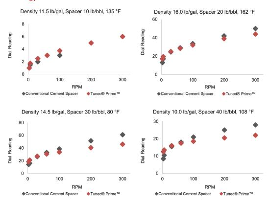
Tuned® Prime™ cement spacers demonstrate comparable rheological behavior to conventional cement spacers over a range of densities, concentrations, and temperatures.
