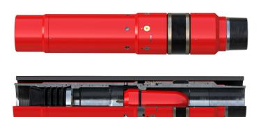
Multiple-Stage Cementing Support > The Obex EcoLock® casing annulus packer provides V6-rated mechanical barrier support to prevent low pressure gas or fluid migration and can support multiple-stage cementing when run as a packer collar with optional integral cementing ports and closing sleeve.
