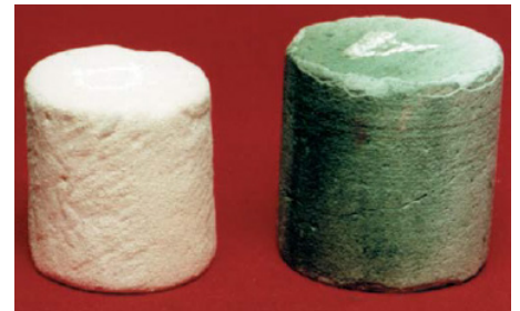
A visual comparison of Portland cement (left) and ThermaLock™ cement (right) shows how CO 2 deteriorates Portland cement over time, while leaving ThermaLock cement virtually unaffected.
