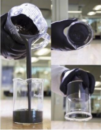
**Curing Losses >** SentinelCem™ cement's rapid static gel strength coupled with early compressive strength helps plug thief zones and mitigate lost circulation.
