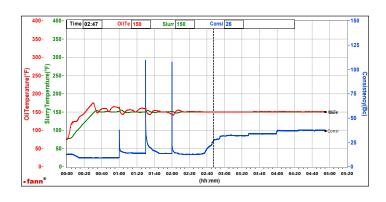
On-off-on testing indicates SentinelCem $^{\text{TM}}$  Pro cement achieves rapid gel strength when shear is removed and regains fluidity for circulation when shear is reapplied.
