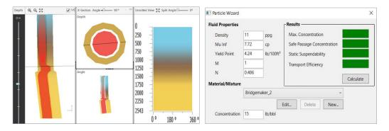
Effective Transport: iCem<sup>®</sup> software helps ensure that the spacer and cement can effectively displace the mud in the annulus in order to create an effective barrier, while Particle Wizard<sup>™</sup> software helps ensure that the spacers and cement can reach the annulus to create the barrier.
