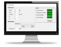
Particle Wizard<sup>™</sup> software evaluates and predicts the ideal material, fluid, and concentration for effective annular clearance. It also accounts for equipment in the well by evaluating depth flow areas and critical flow path dimensions.
