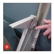
B. If hardware is loose, remove armrest. See 3-6 for proper removal of armrest. Tighten loose hardware and replace any missing or damaged hardware. Reattach the armrest.
