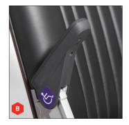
B. Rotate armrest up and down repeatedly. If arm sticks, remove armrest (see 3-6) and inspect rotation pin. Clean area around pin and remove any dirt that may be present. This part requires no additional lubrication.
