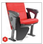
B. Rotate the tablet through its range of motion, and if needed, tighten the torque adjusting nut. This nut is located under the tablet end cap, and regulates the rate at which the tablet goes through its motion. The torque setting on this bolt should be 55 in-lbs (6.2 Nm). Again check to make sure the tablet surface is secured to the mechanism. Hand tighten any loose fasteners, taking care not to strip fasteners. Replace any missing or damaged hardware.
