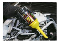
**BG EPR**® is added prior to oil change, dissolves deposits, and is removed with the used oil.
