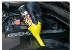
**BG EPR**<sup>®</sup> is added prior to oil change, dissolves deposits, and is removed with the used oil.
