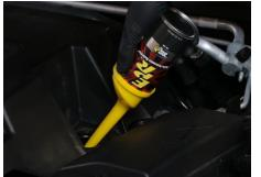
**BG EPR**<sup>®</sup> is added prior to oil change, dissolves deposits, and is removed with the used oil.
