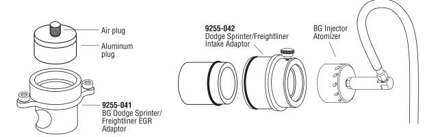
Install aluminum plug into BG Dodge Sprinter/ Freightliner EGR Adaptor
