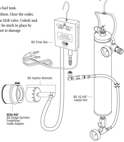
Install BG Dodge Sprinter/Freightliner Intake Adaptor and BG Injector Atomizer
