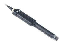
**Important note:** Storing the LDO electrode in alcoholic disinfection solution for more than 16 hours causes visible damage of the LDO sensor cap and its black coating. Consequently the LDO cap can no longer be used for measurements. Similar damages can be seen with the DO membrane cap.
