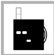
3. Put the tube into the left opening of the color comparator box.
