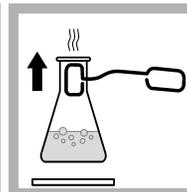
9. Use the clamp to remove the flask.
