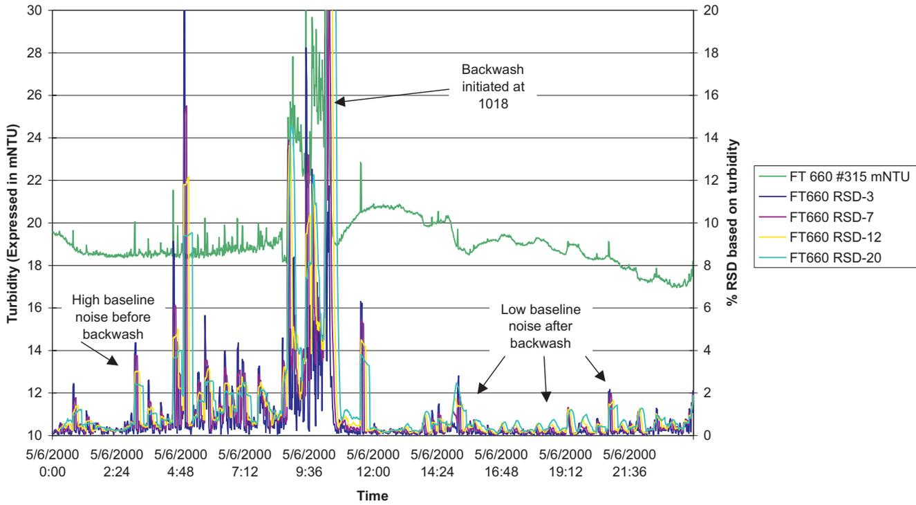
**Figure 7 Filter Run Particle Counts vs. Relative Standard Deviation for WTP Effluent**
