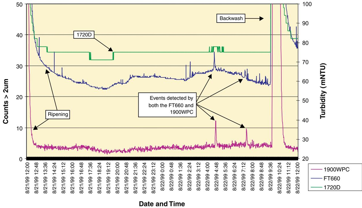
**Figure 10 FilterTrak 660 Typical Filter Run with 1720D Turbidimeter and 1900 WPC Particle Counter Data—Expanded View**
