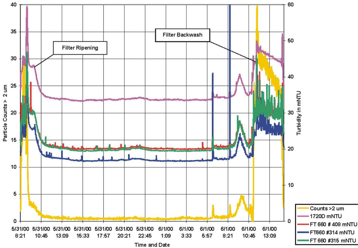
Figure 4 Water Treatment Plant Filter #12 Effluent Particulate Monitoring (06/20/00)
