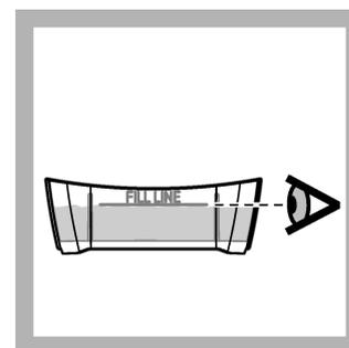
4. Fill the sample cup to the fill-line with sample.
