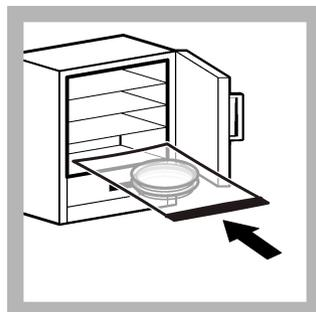
11. Incubate the inverted petri dish at 35 ( $\pm 0.5$ ) °C (95 ( $\pm 0.9$ ) °F) for 48 hours.
