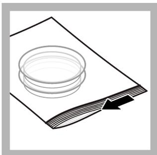
10. Put the inverted petri dish in a plastic bag and seal the bag.
