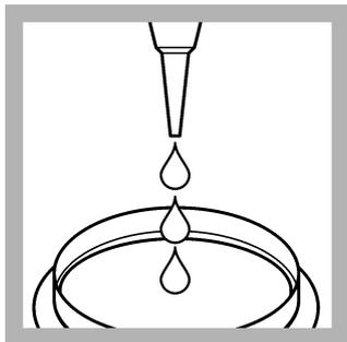
1. Open one m-HPC broth ampule. Lift the lid of a petri dish and carefully pour the contents equally on the absorbent pad.
