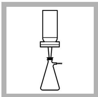
5. Apply the vacuum until the funnel is empty. Stop the vacuum.
