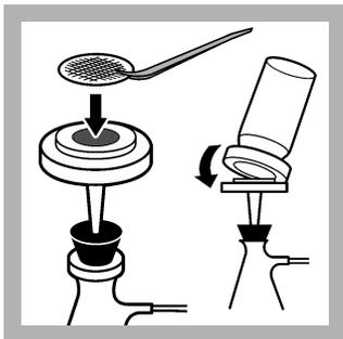
2. Set up the membrane filtration apparatus. Use a sterile forceps to put a membrane filter in the assembly. Make sure that the grid side is up.
