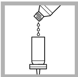
6. Rinse the funnel with 20 to 30-mL of sterile buffered dilution water. Apply the vacuum. Rinse the funnel two more times.
