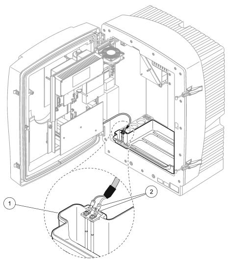
Figure 12 Connect the humidity sensor
