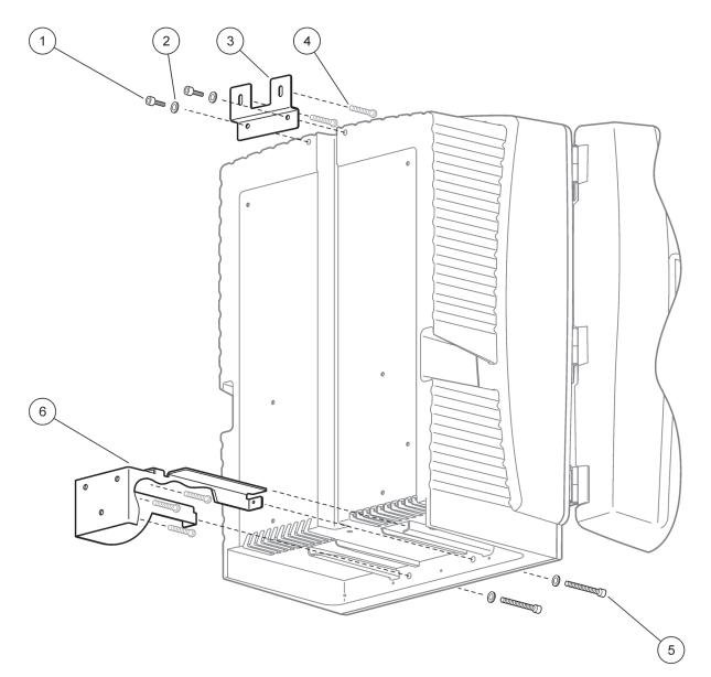
Figure 6 Wall mounting the analyzer
