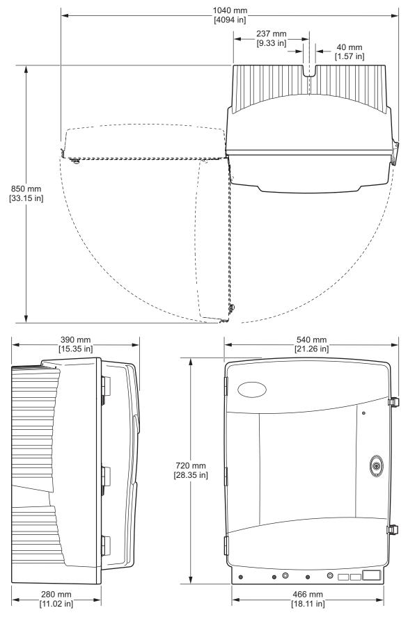
Figure 2 Instrument dimensions PHOSPHAX indoor sc
