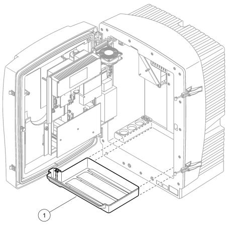
Figure 11 Installation of the collecting tray
