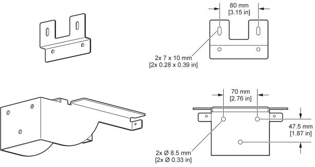
Figure 5 Bracket dimensions for wall mounting
