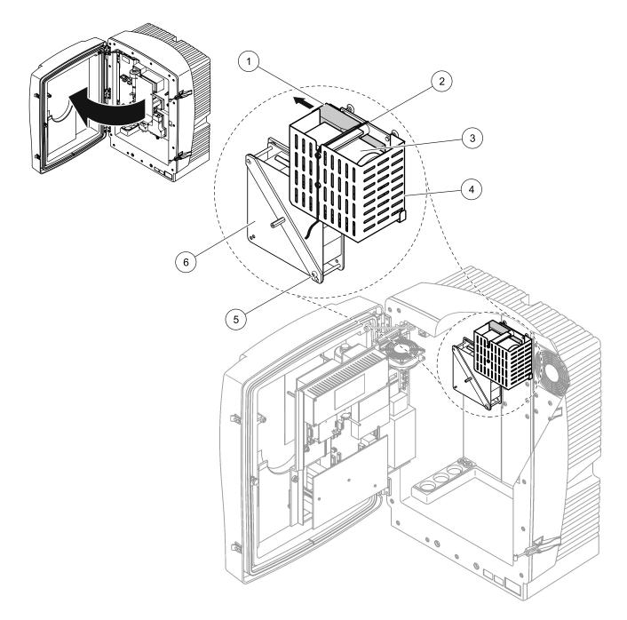
Figure 10 Remove the compressor transport lock<sup>1</sup>
