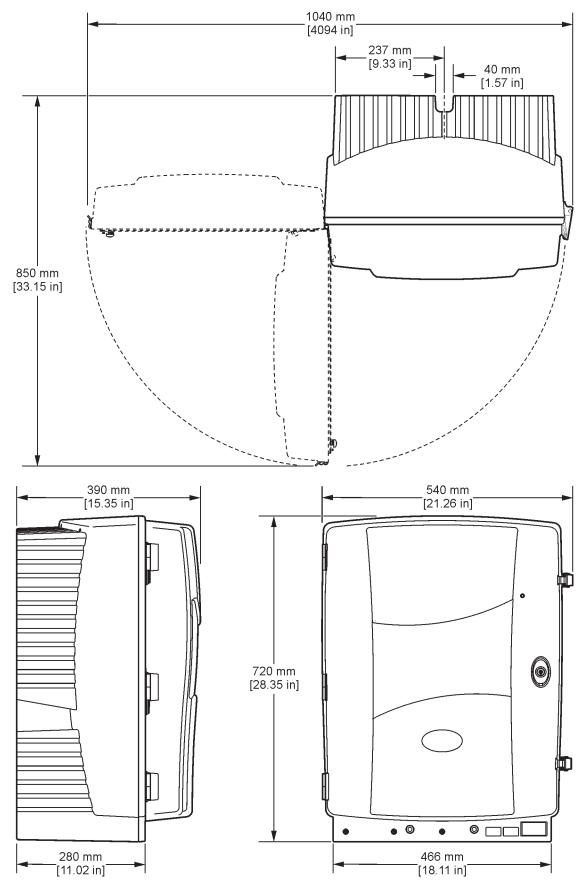
Figure 1 Instrument dimensions PHOSPHAX sc
