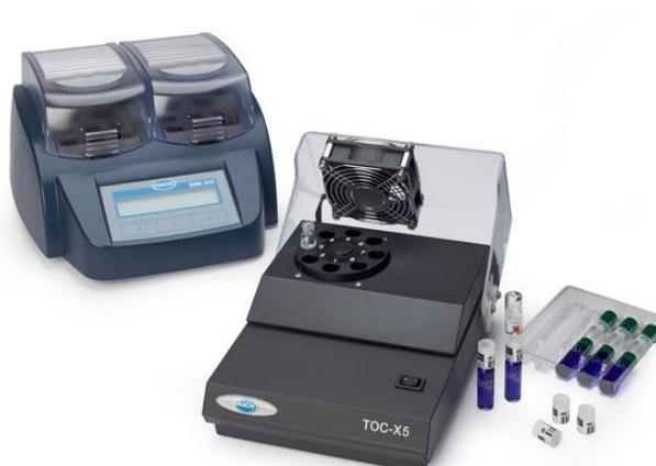
Figure 1: Hach DRB200 reactor, TOC-X5 shaker and TNT+ vials
