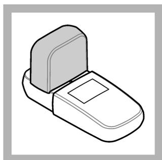
**9.** Install the instrument cap over the cell holder.
