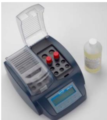
Figure 1: Combination reagent, sample/digestion vials, and digestion block
