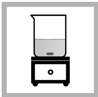
2. Add a stir bar and put the beaker on a magnetic stirrer. Stir at a moderate rate.
