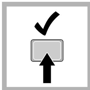
**3.** Push **Read**. A progress bar is shown. When the measurement is stable, the lock icon is shown.
