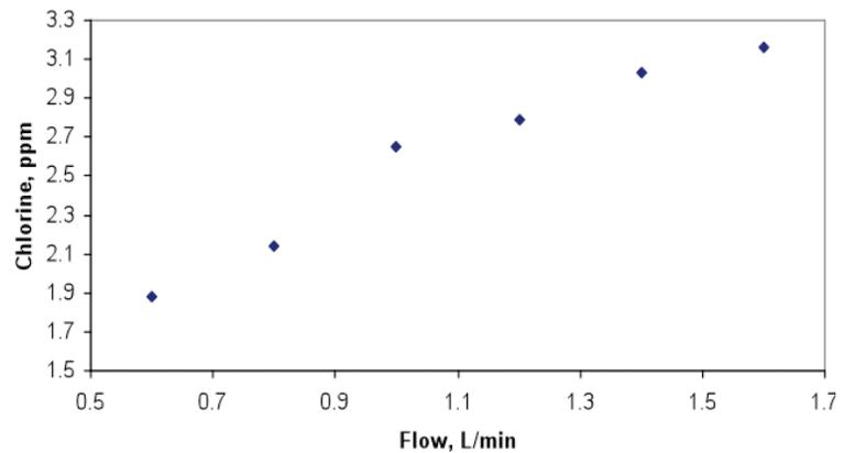
Figure 50: Effect of Flow Rate on an Amperometric Sensor
