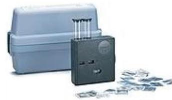
Figure 42: Color Comparator test kit for chlorine residual
