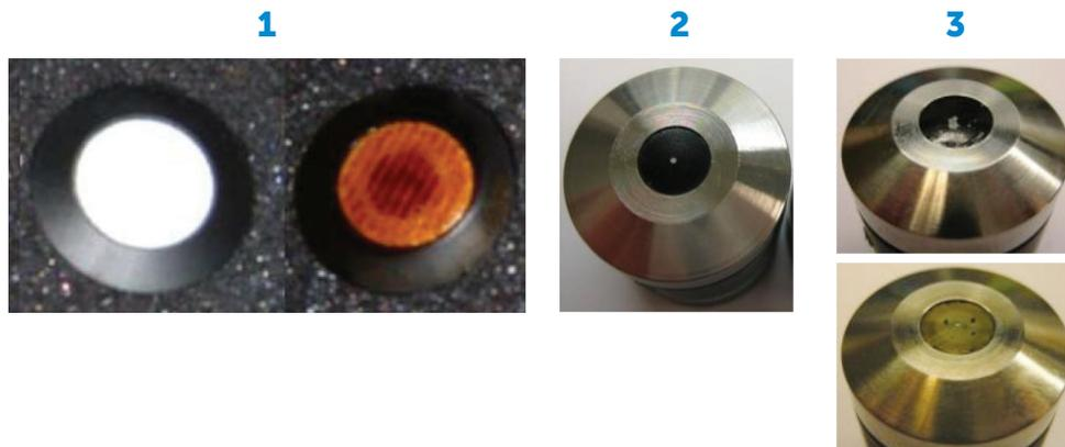
Figure 51: Amperometric probe membranes demonstrating iron fouling and delamination
