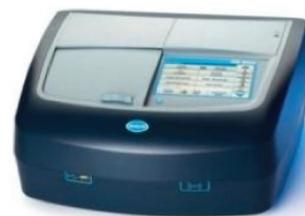
Figure 44: Hach DR6000 UV-Vis Spectrophotometer
