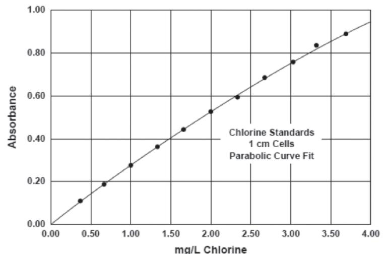
Figure 38: Standard Method Calibration DPD Colorimetric Method
