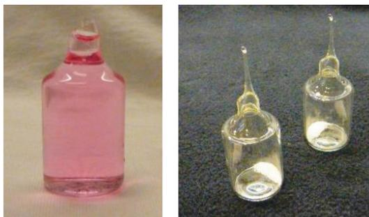
Figure 16: Chlorine residual AccuVac Ampoules
