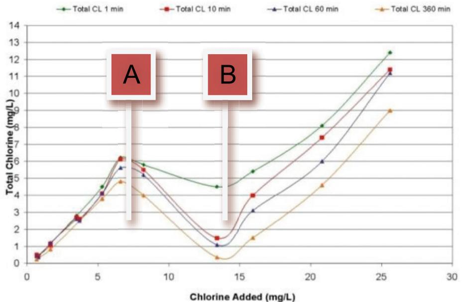
Figure 6: Breakpoint curve due to a significant amount of NOM. Used with permission of the Golden State Water Company.
