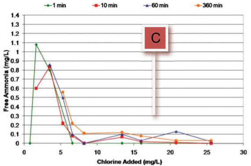
Figure 7: Free ammonia vs. chlorine added. Used with permission of the Golden State Water Company
