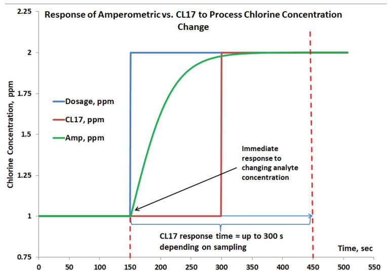
Figure 59: Graphical expression of calculated responses of the CL17 vs. amperometric probe
