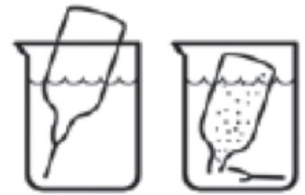
Figure 36: Filling an AccuVac Ampule
