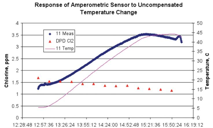
Figure 54: Temperature Effect on an Amperometric Sensor
