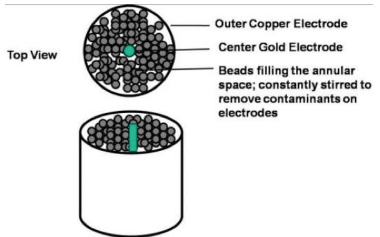
Figure 55: Open-cell amperometric sensor illustration
