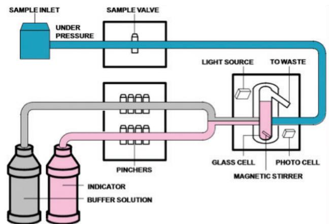
Figure 47: CL17 and CL17sc Flow Path Diagram
