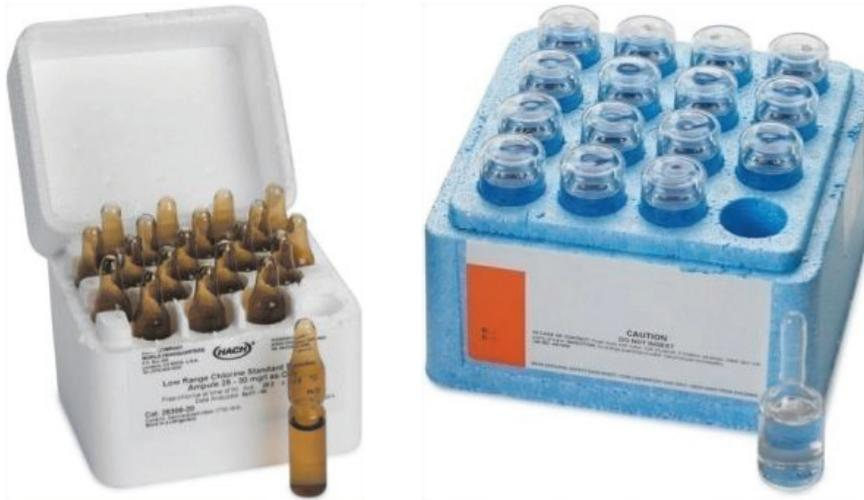
Figure 32: PourRite (left) and Voluette Ampule Chlorine Standard Solutions
