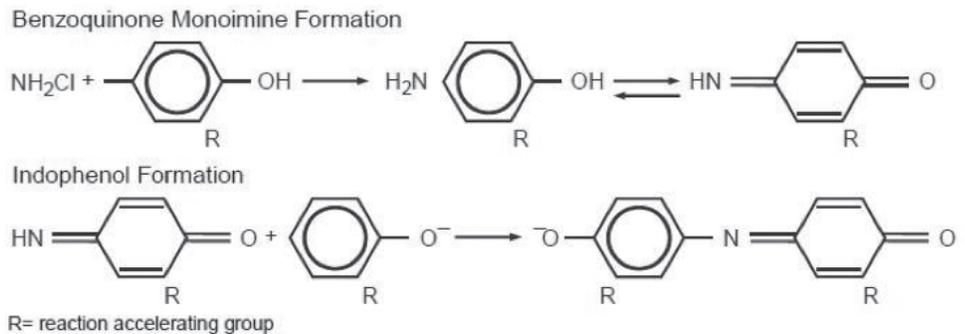
Figure 22: Indophenol formation for determination of monochloramine
