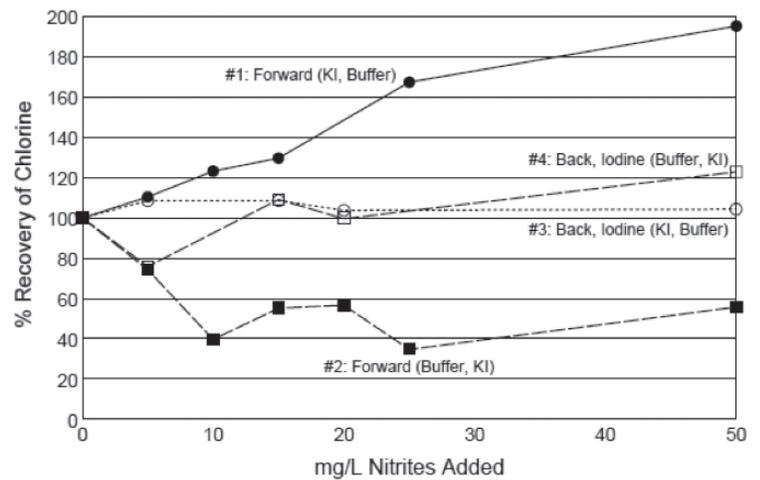
Figure 40: Nitrite interference in amperometric chlorine methods
