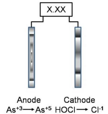
Figure 29: Amperometric forward titration for free residual chlorine
