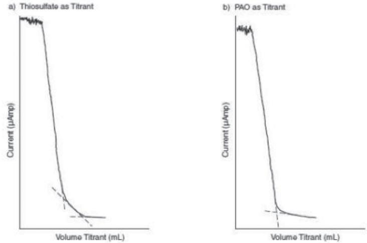
Figure 27: Thiosulfate vs. PAO titrant for amperometric titration
