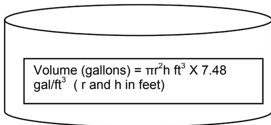
*Note: For a storage tank/reservoir/basin the height or depth MUST be the minimum active level. That is, what is the operational minimum level the tank is permitted to drop to during normal operations on the peak hour of the day? So, if the maximum water depth (height) is 20 ft but the minimum level is 12 feet, then 12 feet must be used in calculation of detention time, T for CT*
