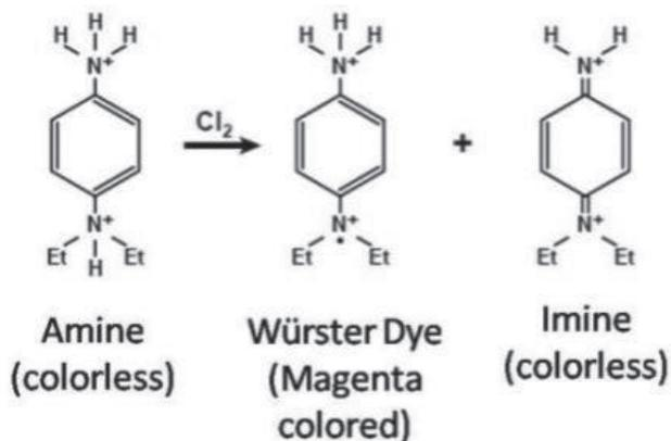
Figure 17: DPD-chlorine reaction products
