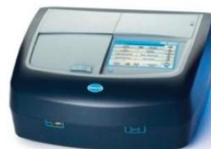
Figure 44: Hach DR6000 UV-Vis Spectrophotometer
