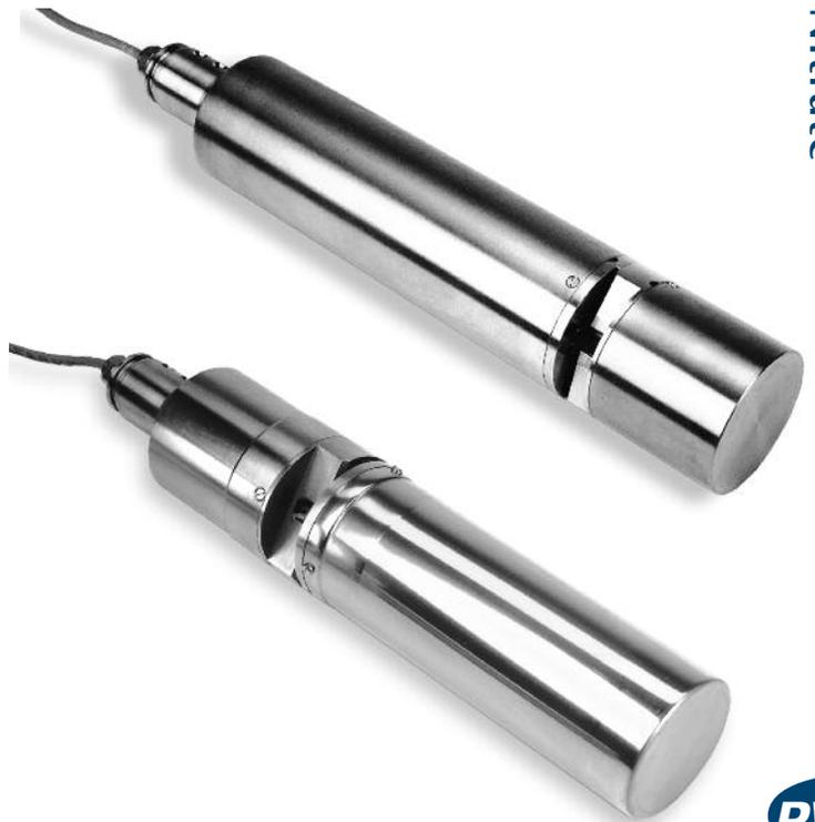
*Sophisticated, yet simple, technology means the Hach NITRATAX sc UV Nitrate Sensors require little maintenance and offers remarkably low cost of operation.*
