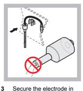
Secure the electrode in the fastening clamp on the front of the panel. Be careful not to touch the membrane.
