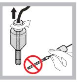
Carefully pull the electrode straight out of the electrode body.
