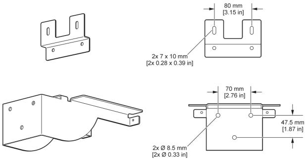
Figure 5 Bracket dimensions for wall mounting
