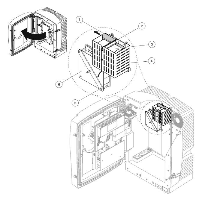
Figure 10 Compressor transport lock removal<sup>1</sup>
