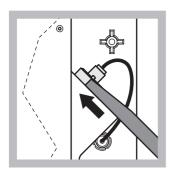
1 Pull the electrode plug. Carefully slide the electrode key under the electrode assembly and pull to remove. Do not apply excessive pressure.
