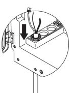
Pull down the plug with the tubing or the cables. Seal any unused entry with Plug #3.
