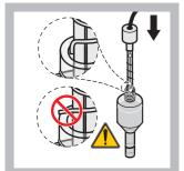
5 Carefully insert the electrode into the body, making sure the electrode tip is not bent.
