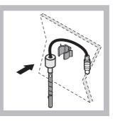
3 Secure the electrode to the clamp on the analyzer panel. Do not touch the membrane.
