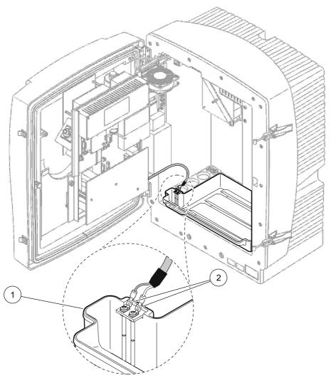
Figure 12 Connect the humidity sensor
