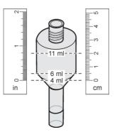
Figure 20 Determine the electrolyte volume in the electrode body with a measuring tape
