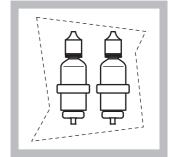
8 Place the bottles of electrolyte into the brackets on the analyzer panel. Close the enclosure door.
