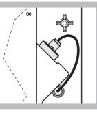
Slide the electrode back into the cell, towards the resistance of the o-ring of the measuring chamber, until it snaps into place and reconnect the electrode cable to the panel.
