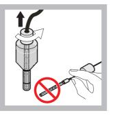
2 Carefully pull the electrode straight out of the electrode body. Do not touch the electrode with fingers. Rinse the glass electrode and the electrode body with distilled water to remove any crystallation that may have occurred, because of complete evaporation.
