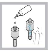
Remove the cap from the electrolyte and fill the body with an entire bottle of electrolyte, (11 mL). Gently tap the side of the body to remove any air bubbles.
