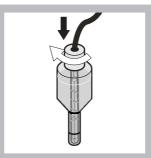
Tighten the sealing cap.
