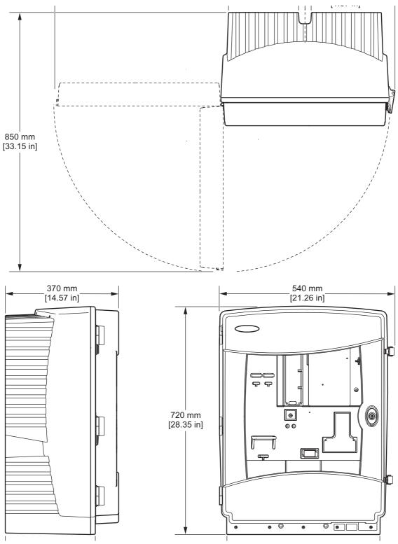
Figure 2 Instrument dimensions AMTAX indoor sc
