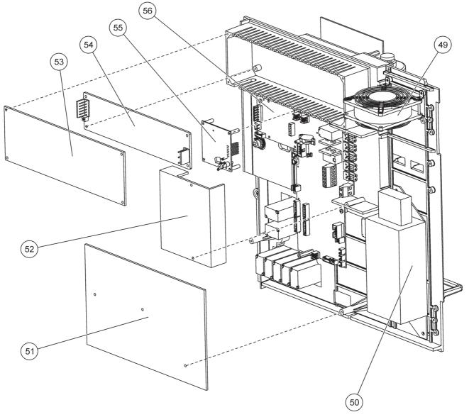
Figure 26 Analyzer panel back view details
