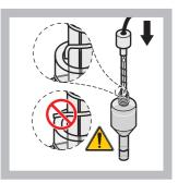
8 Carefully insert the electrode into the body making sure the tip is not bent.
