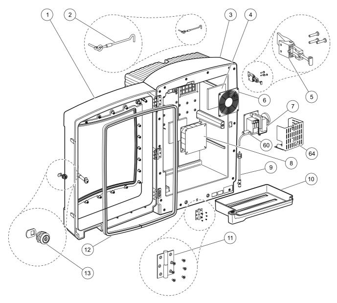
Figure 23 Analyzer enclosure AMTAX indoor sc
