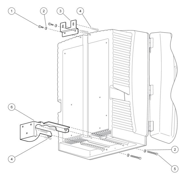
Figure 6 Wall mounting the analyzer
