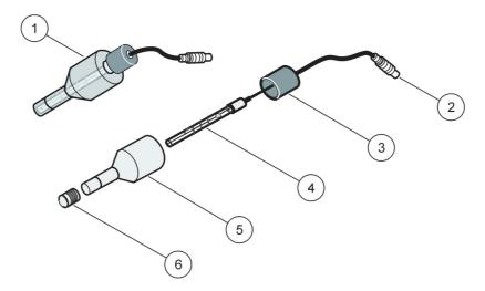
Figure 18 Electrode assembly
