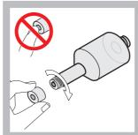
Place the membrane cap on the electrode body. Do not touch the membrane! To prevent the electrolyte from leaking, hand-tighten the electrode cap.
