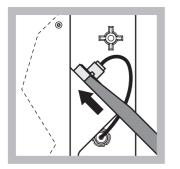
1 Pull the electrode plug. Carefully slide the electrode key (refer to section 8.2, page 67) under the electrode assembly and pull to remove. Do not apply excessive pressure.
