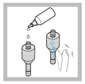
4 Remove the cap from the electrolyte and fill the body with an entire bottle of electrolyte (11 mL). Gently tap the side of the body to remove any air bubbles.
