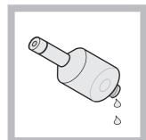
4 Drain the electrolyte from the electrode body.
