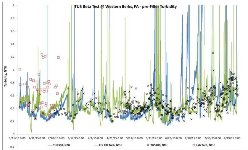
Figure 5: Comparison between turbidity readings from two process and two lab instruments
