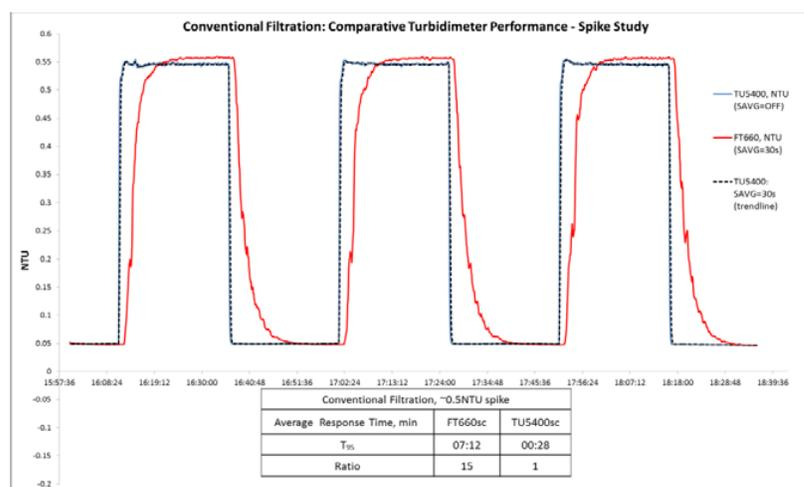
Figure 2: A representative graph and calculations averaging three consecutive spikes to illustrate the response of two turbidimeters measuring conventional filter effluent before and after spiking with Formazin standard
