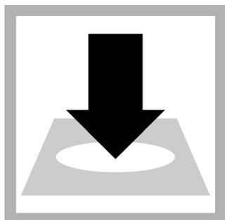
**5.** Insert the blank into the cell holder. Point the diamond mark on the sample cell toward the keypad.
