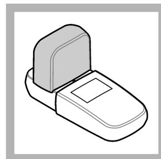
**4.** Install the instrument cap over the cell holder.
