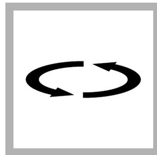
12. Swirl the sample cell for 20 seconds to mix. Do not shake or invert the sample cell. A pink color will show if  $\text{ClO}_2$  is in the sample.
