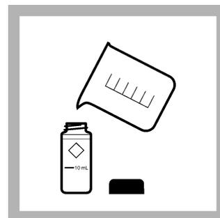
**8. Prepare the sample:** Fill a second sample cell to the 10-mL mark with sample. Complete steps [9–12](#) quickly.
