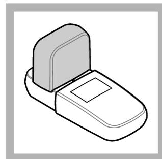
16. Install the instrument cap over the cell holder.
