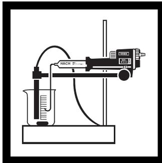
7. Using the Digital Titrator delivery knob, dispense the PAO titrant Solution in 5 to 10 digit increments while noting the downward reading.
