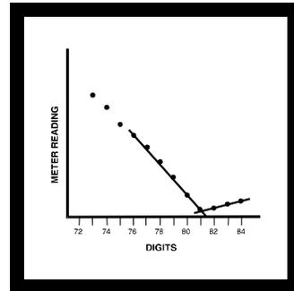
**12.** Draw the two best intersecting lines through the points. Determine the number of digits at the intersection of the lines; this is the end point.
