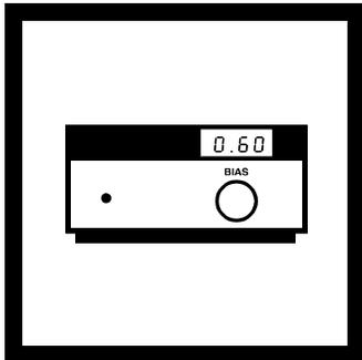
**9.** As the end point approaches, record the LED reading and the corresponding digits on the Digital Titrator. Add a small amount of titrant; wait a few seconds for a stable reading and record.
