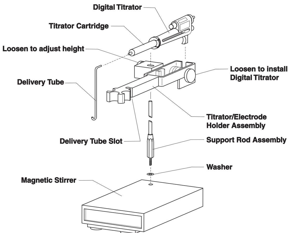
5. Attach the appropriate titration cartridge to the Digital Titrator. Slide the cartridge into the titrator receptacle and lock in position with a quarter turn. Remove the plastic cap from the cartridge tip and insert one of the 90° delivery tubes. Do not insert past the cartridge extension.
