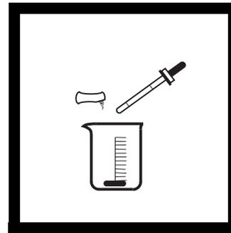
**4.** Add 1 mL of pH 4 Acetate Buffer Solution and the contents of one Potassium Iodide Powder Pillow.
