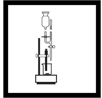
**8.** Continue dispensing slowly. As the end point of the titration is approached, record the LED reading along with the corresponding total volume of titrant added to the nearest 0.01 mL. Add a small amount of titrant; wait a few seconds and record an average value.
