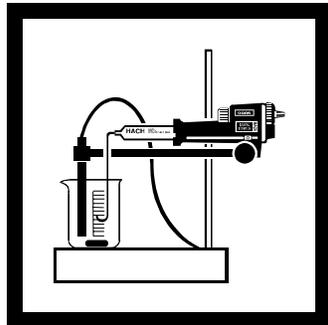
6. Place the beaker on the TitraStir Stir Plate. Turn on the stirring motor. Immerse the tips of the probe and delivery tube into the sample. Make sure the platinum wires are submerged.
