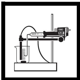
**1.** Assemble the Amperometric Digital Titrator System according to the instructions in *Section 2.2.1* on page 10.
