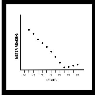
**10.** Plot the recorded readings from the Amperometric Titrator on the vertical axis and the corresponding Digital Titrator digits on the horizontal axis. See *Figure 13*.
