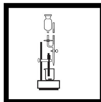
**8.** Continue dispensing slowly. At the end point of the titration is approached, record the LED reading along with the corresponding total volume of titrant added to the nearest 0.01 mL. Add a small amount of titrant; wait a few seconds for a stable reading and record.
