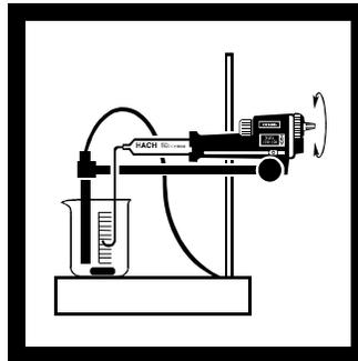
**7.** Using the Digital Titrator delivery knob, dispense the titrant in small increments (5 to 10 digits). The readings on the Amperometric Titrator will decrease.
