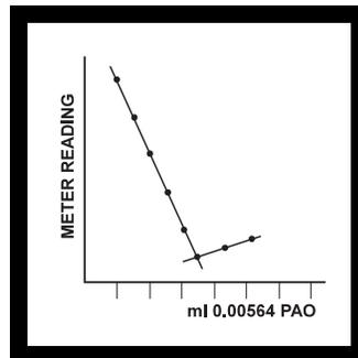
**11.** Draw the two best intersecting lines through the points plotted as shown above. Determine the volume of titrant used to the nearest 0.01 mL at the intersection of the 2 lines. This is the mL Titrant at End Point.
