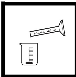
**3.** Without excessive agitation, measure 200 mL sample with a clean graduated cylinder. Transfer the sample to a clean 250-mL beaker containing the 50-mm stirring bar supplied with the system.
