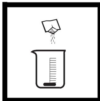
**3.** Add the contents of one Potassium Iodide Powder Pillow. Swirl to dissolve. Place a 50-mm stir bar into the beaker.
