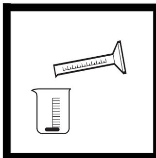
**3.** Without excessive agitation, measure 200 mL of sample with a clean graduated cylinder. Transfer the sample to a clean 250-mL beaker containing the 50-mm stirring bar supplied with the system.
