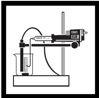
9. Continue the titration, recording at least three points on the downward sloping curve and at least three points after the end point has been reached. The latter points will cause little change in the LED readings.
