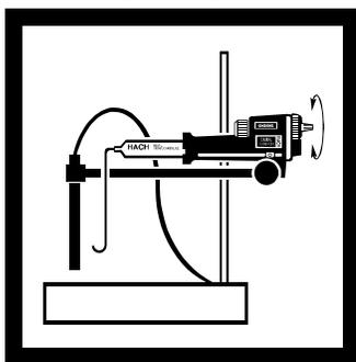
**2.** Assemble the Amperometric Digital Titrator System according to the instructions in *SECTION 2* on page 9. Flush the Digital Titrator delivery tube by turning the delivery knob to eject a few drops of titrant. Reset the counter to zero and wipe the tip.
