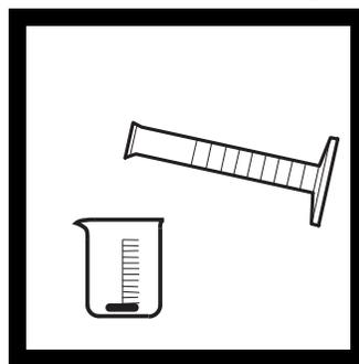
**3.** Place a 50-mm stir bar into a 250-mL beaker. Use a graduated cylinder to transfer 200 mL of sample to the beaker.
