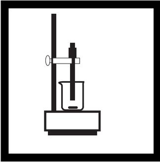
**5.** Place the beaker of prepared sample on the TitraStir Stir Plate and turn on the stirring motor. Immerse the tip of the probe in the prepared sample. The platinum wires must be submerged.
