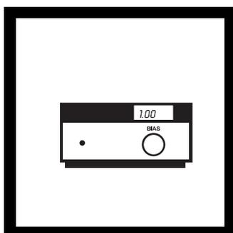
**6.** Note the LED reading on the Amperometric Titrator. Using the BIAS control, adjust the LED reading to about 1.00.
