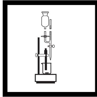
**7.** Dispense the titrant into the beaker in small increments while observing the downward readings on the Amperometric Titrator.
