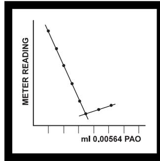
**11.** Draw the two best intersecting lines through points plotted as shown above. Determine the volume of titrant used to the nearest 0.01 mL at the intersection of the two lines. This is the mL titrant at End Point.
