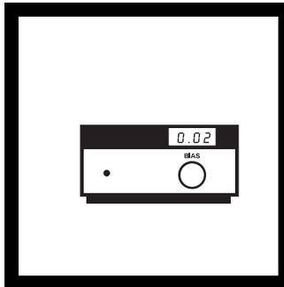
7. Note the LED reading on the Amperometric Titrator. Unlock the BIAS control and adjust the BIAS control knob until a reading between 0.50-0.60 is obtained. Lock the BIAS control.
