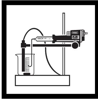
**10.** Continue the titration, recording at least three points on the downward sloping curve and at least three points after the end point has been reached. The latter points will cause little change in the LED readings.
