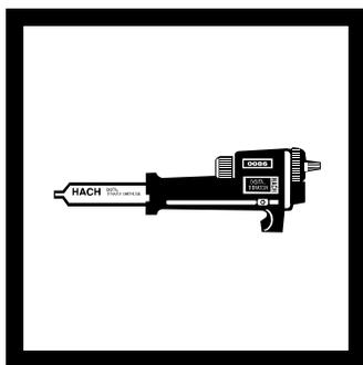
**1.** Install the 0.0451 N Phenylarsine Oxide Titration Cartridge (PAO) on the Digital Titrator.
