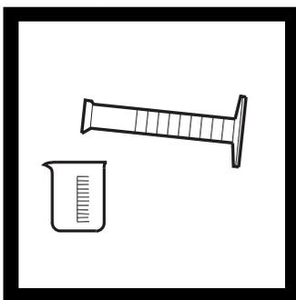
**2.** Use a graduated cylinder to measure 200 mL of sample. Transfer to a 250-mL beaker.
