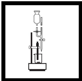
**9.** Continue the titration by recording at least three points on the downward sloping curve and at least three points after the end point has been reached. The latter points will indicate little change in the meter readings.
