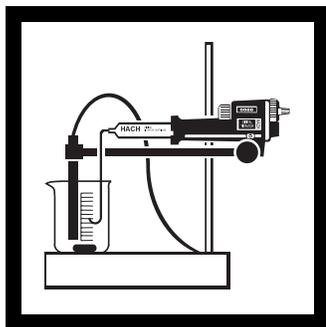
**6.** Using the Digital Titrator delivery knob, add 50 digits of Standard Iodine Titrant Solution.
