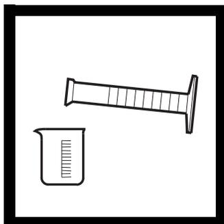
**2.** Use a graduated cylinder to measure 200 mL sample into a 250-mL beaker.
