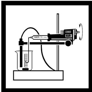
**10.** Continue the titration. Record at least three points on the downward sloping curve and at least three points after the end point has been reached. The last three points will show very little change in the meter readings.
