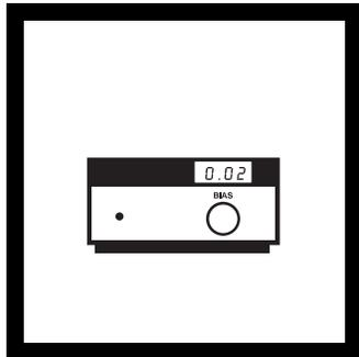
6. Note the LED reading on the Amperometric Titrator. Unlock the BIAS control and adjust the BIAS control knob until a reading between 0.50-0.60 is obtained. Lock the BIAS control.
