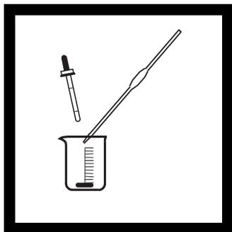
**2.** Place a clean 50-mm stirring bar supplied with the system into a clean 250-mL beaker. Using a Class A pipet, transfer 1.00 mL of 0.00564 N Sodium Thiosulfate Solution to the a beaker. Add 1 mL of pH 4 Acetate Buffer Solution to the beaker.
