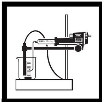
7. Using the Digital Titrator delivery knob, dispense 100 digits of Standard Iodine Titrant Solution and note the LED reading.
