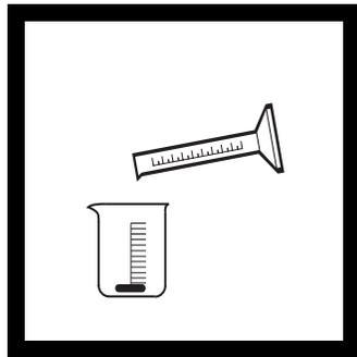
**2.** Using a graduated cylinder, measure 200 mL of deionized water into a clean 250-mL beaker. Place the 50-mm stirring bar supplied with the system into the beaker.
