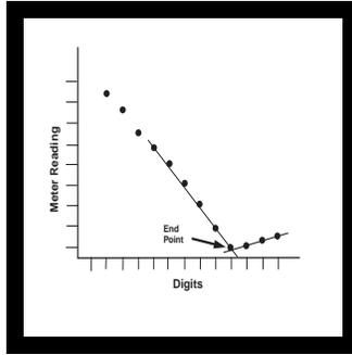
**11.** Using linear graph paper, plot the recorded readings from the Amperometric Titrator on the vertical axis and the corresponding Digital Titrator digits on the horizontal axis. Draw the two best intersecting lines through the points (see *Figure 15*). Determine the number of digits at the intersection of the lines; this is the end point.
