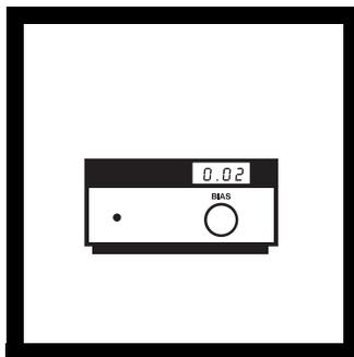
**7.** Note the LED reading on the Amperometric Titrator. Unlock the BIAS control and adjust the BIAS control knob until a stable reading between 0.50-0.60 is obtained. Lock the BIAS control.
