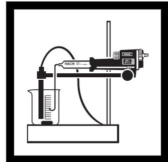
8. Using the Digital Titrator delivery knob, dispense the PAO titrant Solution in 5 to 10 digit increments while noting the downward reading.
