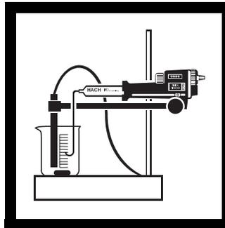
7. Using the Digital Titrator delivery knob, dispense the Standard Iodine Titrant Solution in 5 to 10 digit increments while noting the reading. Record at least three points (the null current values and Digital Titrator reading), before end point is reached.
