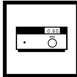
**8.** As the end point approaches, record the LED reading and the corresponding digits on the Digital Titrator. Add a small amount of titrant; wait a few seconds for a stable reading and record the reading.
