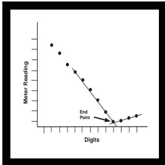
10. Using linear graph paper, plot the recorded readings from the Amperometric Titrator on the vertical axis and the corresponding Digital Titrator digits on the horizontal axis. Draw the two best intersecting lines through the points; see *Figure 12*. Determine the number of digits at the intersection of the lines; this is the end point.
