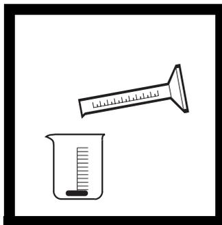
**3.** With minimum agitation, measure 200 mL of sample with a clean graduated cylinder and transfer the sample to the beaker. Swirl to mix the reagents with sample.
