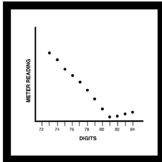
**11.** Using linear graph paper, plot the recorded readings from the Amperometric Titrator on the vertical axis and the corresponding Digital Titrator digits on the horizontal axis. See *Figure 13* on page 41.
