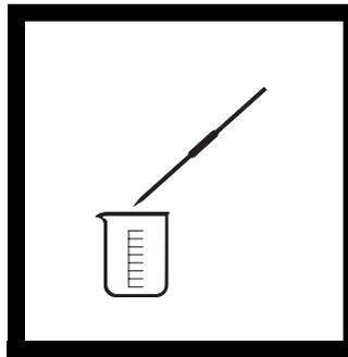
**3.** Using a Class A pipet, transfer 1.00 mL of 0.00564 N Sodium Thiosulfate Solution to the beaker. Swirl to mix.
