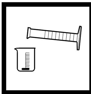
**3.** Without excessive agitation, measure 200 mL of sample with a clean graduated cylinder. Transfer the sample to a clean 250-mL beaker containing the 50-mm stirring bar supplied with the system.
