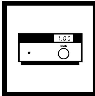
7. Note the LED reading. Use the BIAS control to adjust the LED reading to about 1.00.
