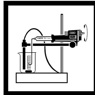
8. Using the Digital Titrator delivery knob, dispense the titrant in small increments (5 to 10 digits). The readings on the Amperometric Titrator will decrease.
