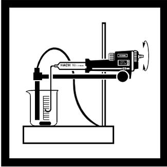
**9.** Continue the titration. Record at least three points on the downward sloping curve and at least three points after the end point has been reached. The last three points will show very little change in the meter readings.
