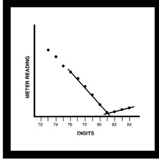
**11.** Draw the two best-fit intersecting lines through the points. Determine the number of digits at the intersection of the lines; this is the end point.
