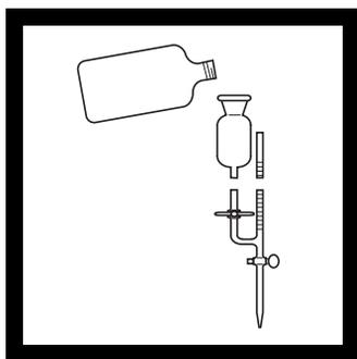
**1.** Fill the 5-mL automatic buret to the zero mark with 0.00564 N Phenylarsine Oxide (PAO) Solution.
