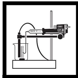
**4.** Place the beaker on the TitraStir Stir Plate and immerse the tips of the probe and delivery tube in the solution. The probe's platinum wires must be submerged. Turn on the stirring motor.
