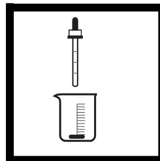
**4.** Add 1.0 mL of pH 4 Acetate Buffer Solution to make the prepared sample.
