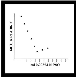
**10.** Construct a graph of the titration by plotting the readings obtained from the Amperometric Titrator display on the vertical axis and the corresponding volume of titrant used on the horizontal axis.
