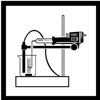
**5.** Place the beaker on the TitraStir Stir Plate. Turn on the stirring motor. Immerse the tips of the probe and delivery tube into the sample. Make sure the platinum wires are submerged.
