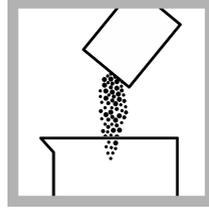
3. Add one Fluoride Ionic Strength Adjustor (ISA) Powder Pillow to each 25 mL of standard solution.
