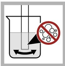
7. Shake the probe from side to side to remove air bubbles.
