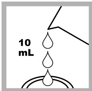
2. Fill a sample cell with 10 mL of sample.
