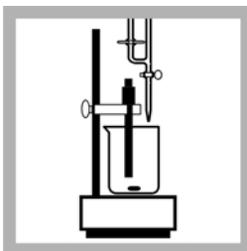
7. Dispense the titrant into the beaker in small increments while monitoring the values on the Amperometric Titrator. The values will decrease.
