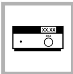
6. Turn the BIAS control knob to adjust the value on the display to approximately 1.00. The BIAS adjustment controls the slope of the titration curve. The actual value is not important. Only the relative value as the titration continues is important. A precise adjustment is not necessary.
