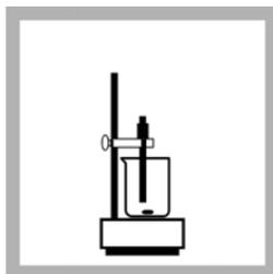
5. Place the beaker of prepared sample on the TitraStir titration stand and turn on the stirring motor. Put the tip of the probe fully into the prepared sample. The platinum wires must be submerged. If a stir plate other than the TitraStir® is used, set the speed for moderate mixing. Do not adjust the speed after this point.
