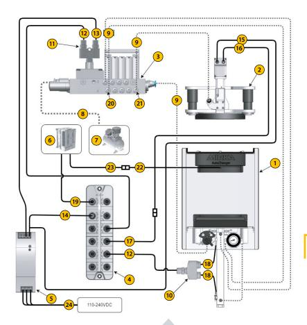
The simplified connection chart gives the integrator an overview of how the AutoChanger modules are supposed to be connected.
