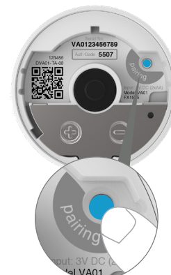
Press the button for 3s to activate pairing
