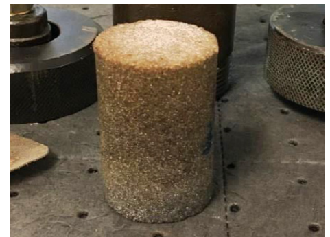
FineStop™ C service stops the migration of damaging fines by providing consolidation strength to the formation grains
