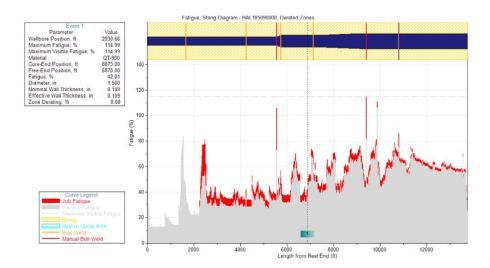
Above » Extensive testing and field evaluations have proven the consistency and reliability of Halliburton's fatigue life model which takes into account factors including job exposure type (acid, H<sub>2</sub>S, CO<sub>2</sub>, etc.), internal and external pressures, ovality, and the number of cycles.
