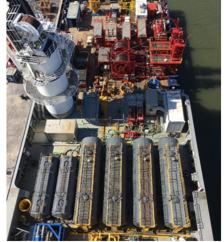
Dual downline installation on the deck of a vessel
