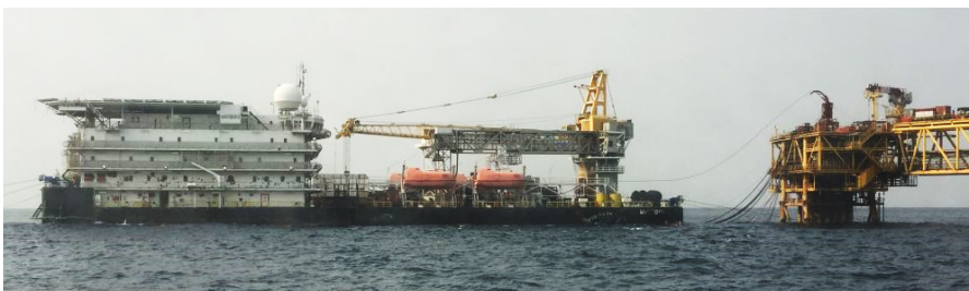
Example of a catenary CT rig-up
