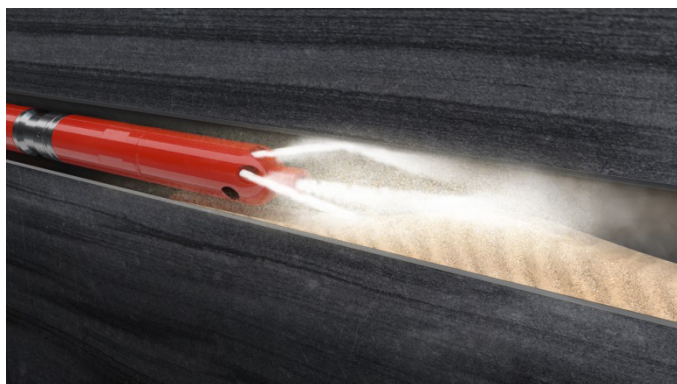
SandKleen® High Pressure Jetting Mode uses powerful forward jets to fluidize sand bridges and return settled fill into suspension.
