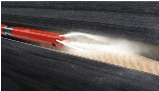
SandKleen SM High Pressure Jetting Mode uses powerful forward jets to fluidize sand bridges and return settled fill into suspension.
