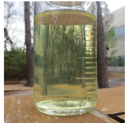
ZCA™ II is a non-polymeric acid gelling agent used to enable self-diverting acid treatments
