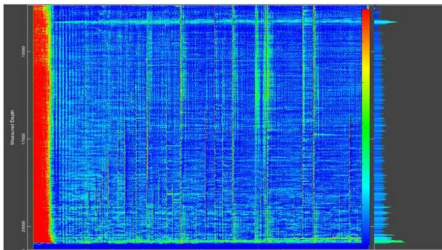
Figure 8—DAS signal during well open; no significant anomaly, 17,100 ft
