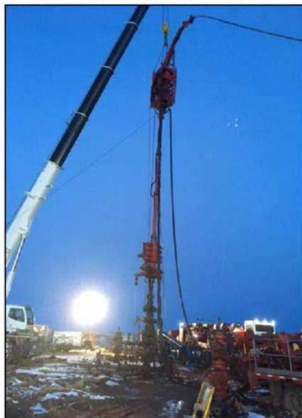
Figure 2—2 3/8-in. CT fiber-optic unit injector head and pressure control stack.
