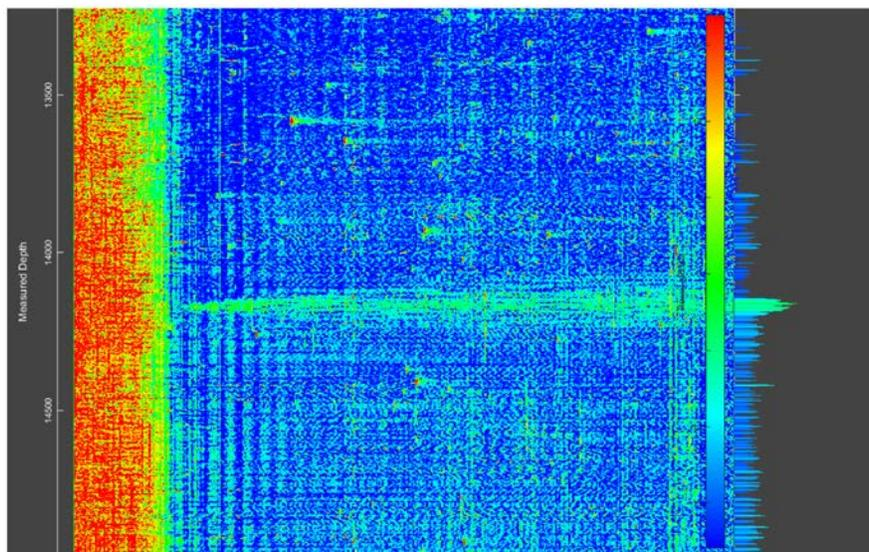
Figure 7—DAS signal during well open with lowpass filter.
