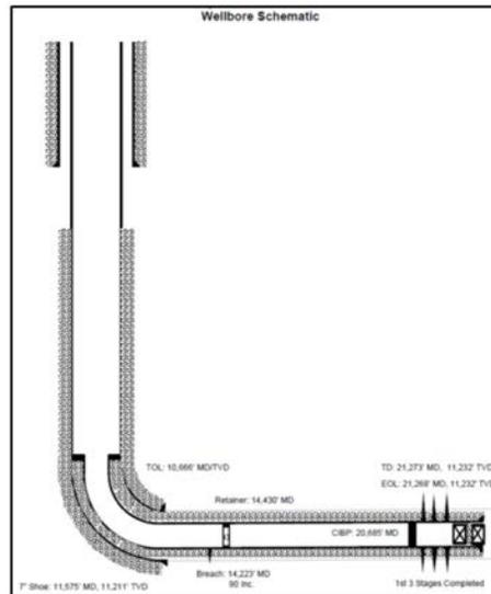
Figure 1—Simplified wellbore schematic.
