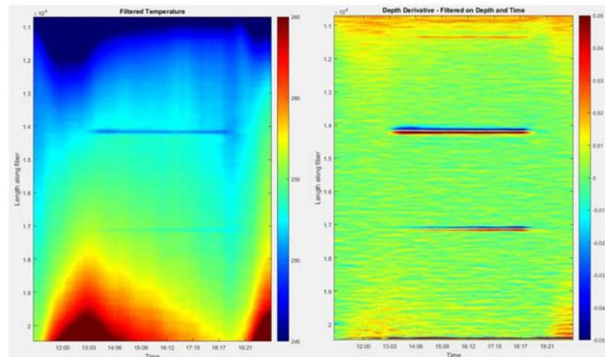
Figure 6—DTS depth derivative lateral section; filtered data set.
